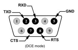
Figure 3-14: Rear Panel Connector Pin-Outs for RS-232 Mode
